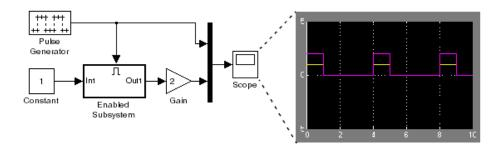
Simulink software computes the outputs of the Constant block and Gain Block only when the Enabled Subsystem executes (i.e., at time steps 0, 4, 8, and so on). This is because the output of the Constant block is required and the input of the Gain block changes only when the Enabled Subsystem executes. When CE behavior is off, Simulink software computes the outputs of the Constant and Gain blocks at every time step, regardless of whether the outputs are needed or change.
